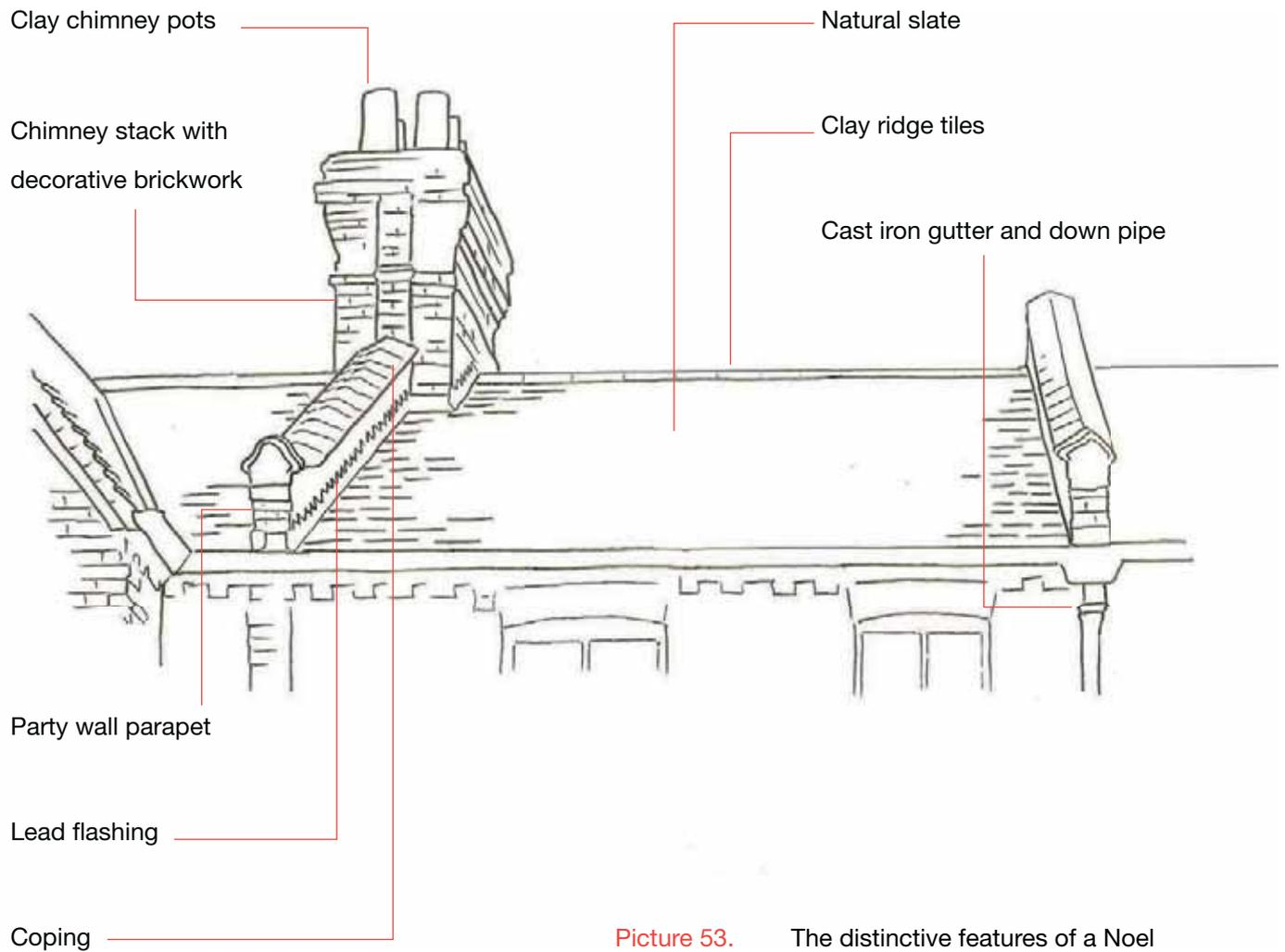
**Picture 53.** The distinctive features of a Noel Park roof, which should be retained, repaired and reinstated
