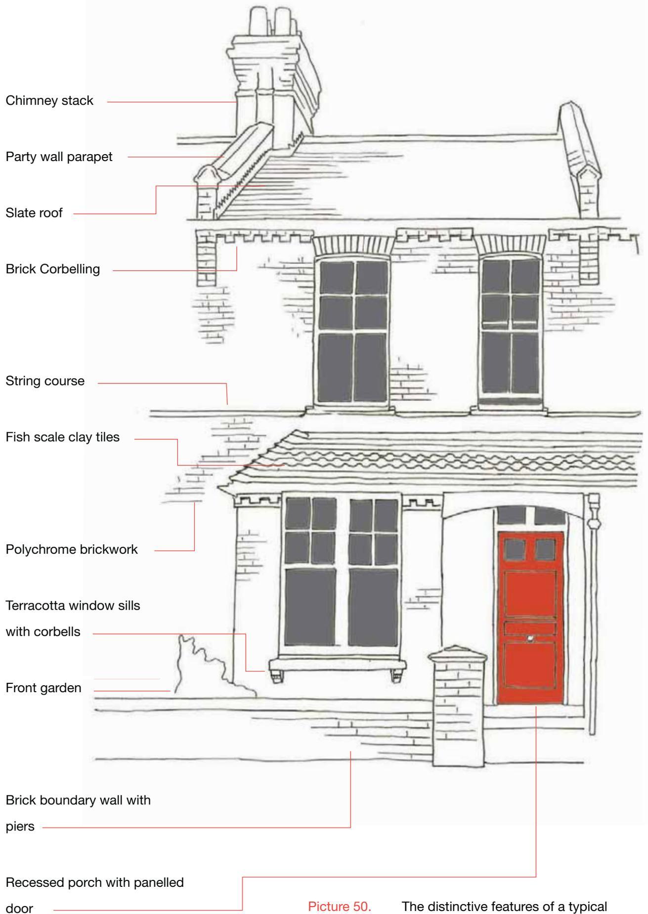
**Picture 50.** The distinctive features of a typical Noel Park house which should be retained, repaired or reinstated wherever possible.
