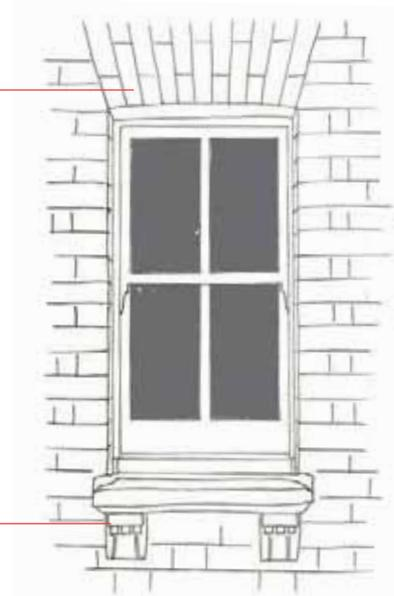
**Picture 51.** The features of typical Noel Park windows, which should be retained, repaired or reinstated where possible.
